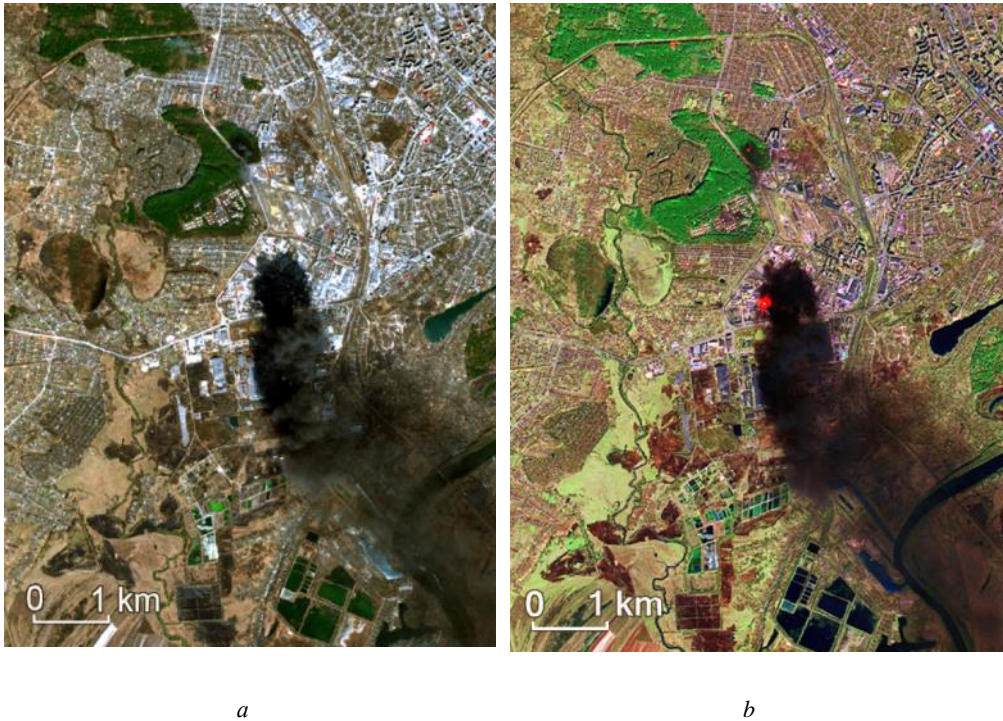
Fig. 3: Image of the fire at the oil depot in the south-western part of Chernihiv according to Sentinel 2B satellite from March 23, 2022: a – by combinations of channels of the visible spectrum, b – using the infrared channel B11.
