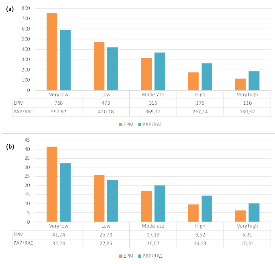
Fig. 7: Diagram of erosion intensity according to EPM and PAP/RAC models by area in m^3/km^2/y (A) and in percentage (B)
